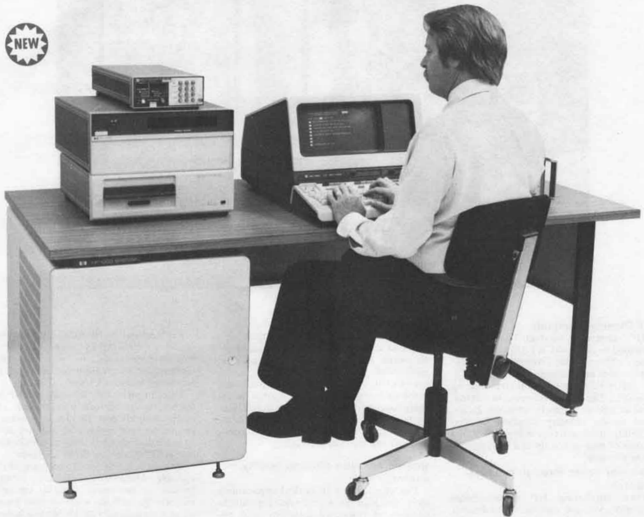
HP 1000 Model 20 Computer System with HP-IB instruments and optional Flexible Disc
