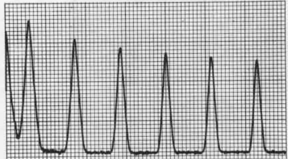
Figure 5a. This represents a portion of a frequency multiplexed system operating normally. Notice that not all channels are operating at the same level.
