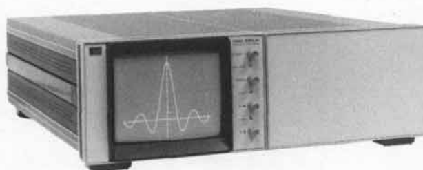
1340A Option 315 installed in 10380A cabinet
