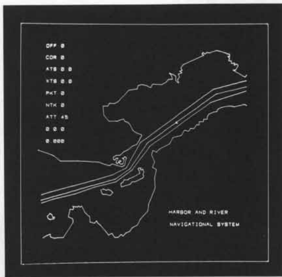
Harbor and river navigational radar systems: the harbor, shoreline, and labeling can be placed in different memory files from ship location, velocity, and direction vectors. If a particular ship is in potential danger, parameters can be made to flash for emphasis.
